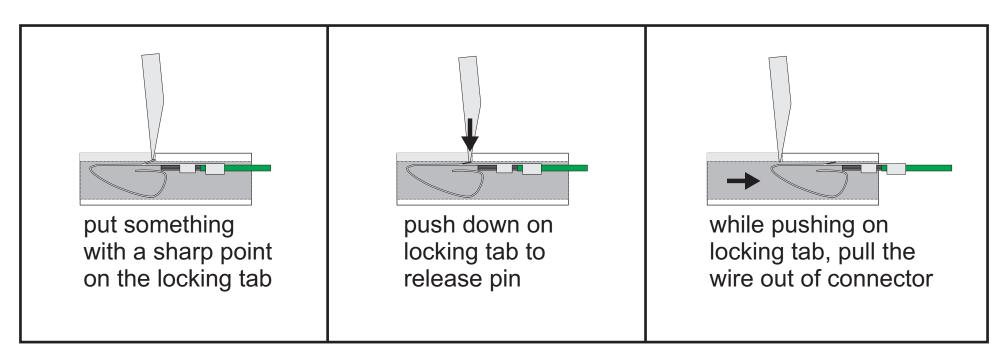
to insert wire, simply reverse the above process, making sure the locking tab is pointed up toward the slot in the connector so it will lock into place.
